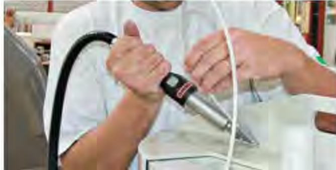
Draw welding using the compact and light Masa WELDING PEN R.
